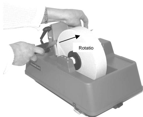
**NOTE!** Before you start grinding make sure the stone rotates in the right direction (pic. 2)
